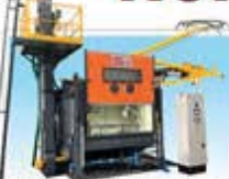
Spl. Blasting M/c for Roof-Mounted Parapets Contact Strips of Electric Rail
