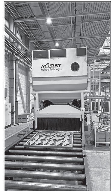
At a distance between rollers of 400 mm, the roller conveyor allows the treatment of work pieces with lengths of at least 1,500 mm. With a special transport frame smaller work pieces can be handled easily
