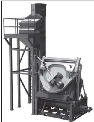
The drum of the Multi-Tumbler blast machine, with its pyramid-shaped bottom and special ribs on the inner wall, has no gaps, where the work pieces might get lodged and damaged. Therefore, this machine type is ideal for processing small and very small work pieces
