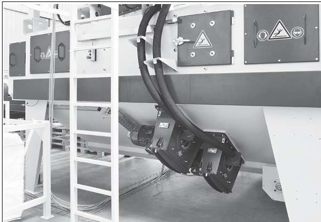
The blast performance and placement of the six turbines – three blast from the top and three from below – ensure that the required shot blasting results are consistently achieved with non-abrasive round steel shot
