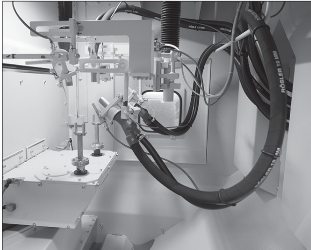
The blast nozzles, placed at the top and bottom of a vertical linear shuttle unit, can be moved up/down and individually turned on or off
